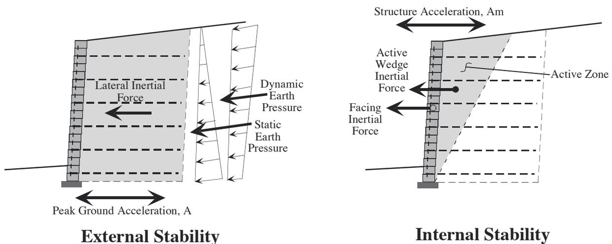
A seismic design must evaluate the combined loading condition of static, dynamic, and inertial forces acting on the structure, both externally and internally, and provide sufficient resistance to mitigate failure during the design event. It is customary to utilize 75% of the normal static design safety factors (ie; 75% of 1.5 min = 1.1 min) for the combined loading condition analysis.
